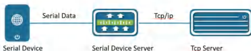
Figure 3-53 Serial device server work in tcp-client mode
